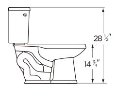
THIS FIXTURE QUALIFIES ACCORDING TO ASME TEST PROCEDURES AS A LOW CONSUMPTION WATER CLOSET WITH AN AVERAGE CONSUMPTION OF 1.6 GAL. OR LESS.
