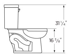
THIS FIXTURE QUALIFIES ACCORDING TO ASME TEST PROCEDURES AS A WATER CLOSET WITH AN AVERAGE CONSUMPTION OF 1.6 GAL. OR LESS.
